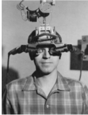
Figure 37: Engineer Ivan Sutherland wearing head-mounted display, 1970
