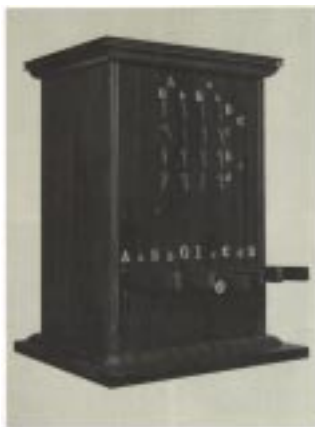
Figure 4: Marquand's Logic Machine
