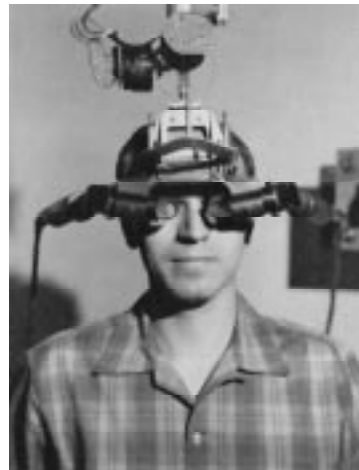
Figure 2.61: Engineer Ivan Sutherland wearing head-mounted display, 1970
