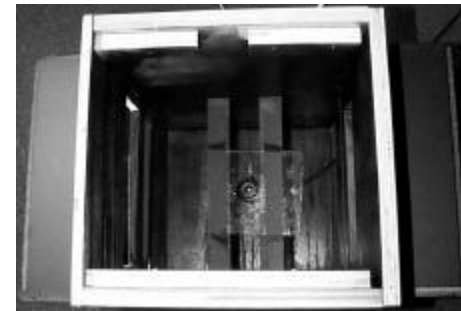
Inside of final input pad. The long lights along the left and right light the underside of the bladder (here removed) evenly, but are placed high enough so that their reflection cannot be seen by the camera.
