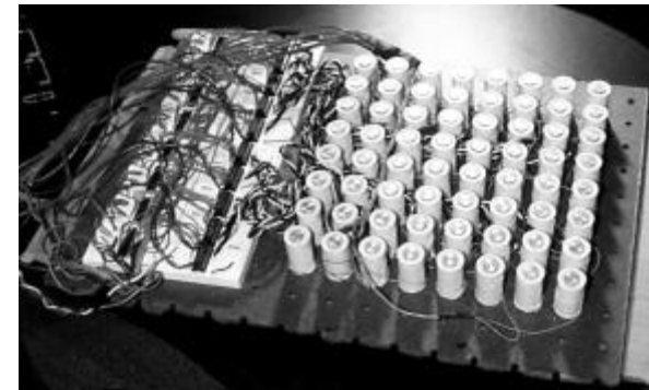
Magnetic grid under output pad
