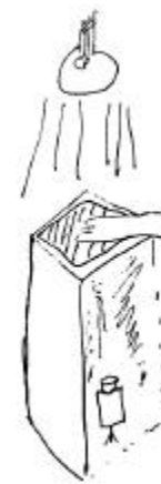
Sketch of initial prototype where light from above is transmitted through the liquid to the camera below in the box when the pad is compressed.
