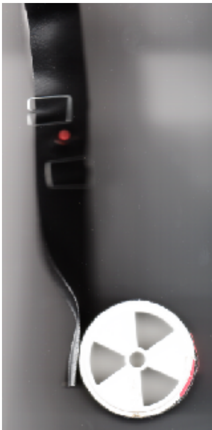
Problem 2 Measuring Tape in Nylon. This 4ft linear device digitally records the distance that it has been unwound. The tape is embedded with pressure sensors which are depressed while the device is rolled up. As these sensors are released, they trigger hotpants to graphically represent the portion of tape which has been unraveled.
