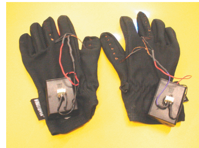
6.4.2 Light gloves show palm down exposing battery pack
