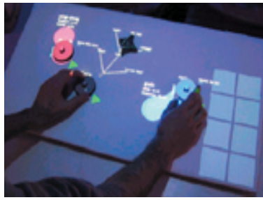
2.3.9 overhead view of entire AudioPad interface
