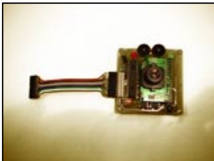
Figure #: A standalone camera board turns LittleVision into a self-contained tiny videocamera.
