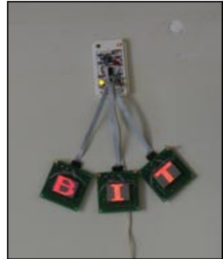
Figure #: Word Toss handhelds sending information over a visible laser.
