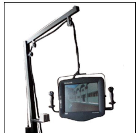
Figure #: The WindowsVR rig has joysticks to register translation. [Absolut, 2002]
