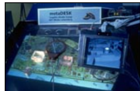
Figure #: Brygg Ullmer's metaDESK uses a variety of physical tools and metaphors to allow users to interact with geographical data.
