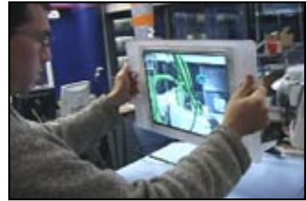
Figure #: Moving the viewscreen around causes the forms to react as if they were exactly where they were placed in the room.
