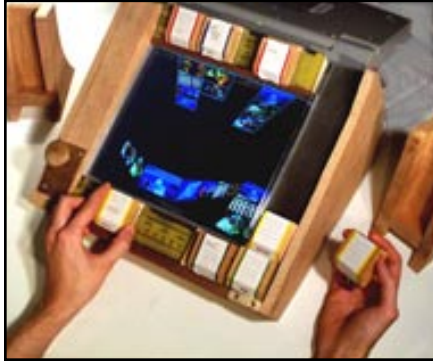
Figure #: Brygg Ullmer's mediaBlocks lets users store and manipulate media clips as if they were stored in wooden blocks.
