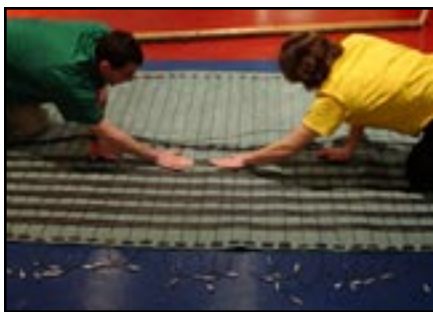
Figure #: Rewiring the carpet with piezoelectric wires. [Photo by Stephanie Hunt].
