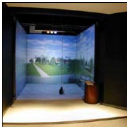
Figure #: A VR "CAVE" projects 10' X 10' images on four sides. [http://www.eds.com/services_offerings/vr/centers_the_way.shtml]
