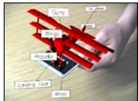
Figure #: The ARToolkit is used to composite a virtual plane into a video image. [http://www.equator.ecs.soton.ac.uk/projects/arproject/fokker-ar.jpg]
