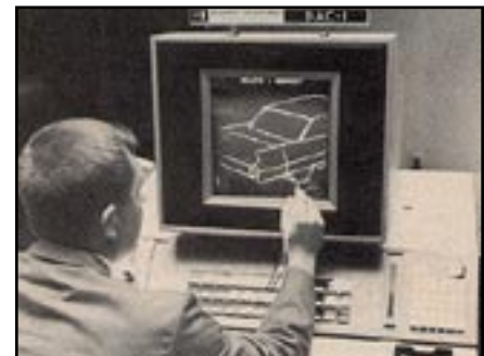
Figure #: In 1959, the DAC-1 (Design Augmented by Computers), developed by General Motors and IBM, was the first interactive 3D computer graphics system.
