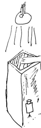
Sketch of initial prototype where light from above is transmitted through the liquid to the camera below in the box when the pad is compressed.
